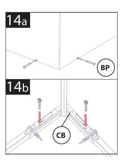
Push base pins into holes in the bottom edge of outer panels and through corner bracket (a). Anchor box to timber base frame as shown or concrete slab / other flat surface (b). Do this for for all 4 corners.
