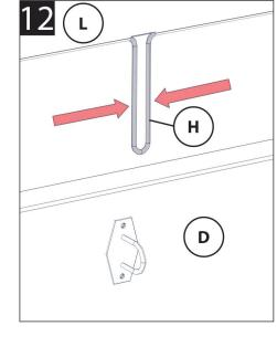
Insert staple into slot into top lid by pinching sides.
