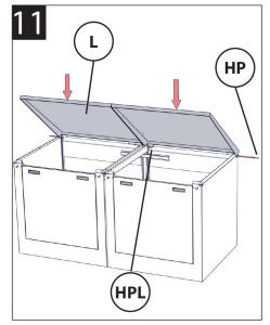
Attach the lids to unit with hinge pins. "click" is heard. Place the removable front Align pins with holes and tap into place with a mallet. For the central join, tap the
