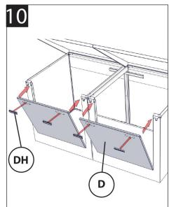
door into the panel by placing the lip of the door over the front panel step. Insert centre hinge pin through both top lids the door by aligning the studs on the side and corner caps. with the slots in the front panel. Push in slightly and then down.
