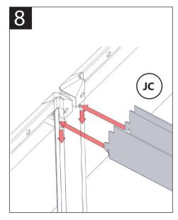
Now it's time to attach the joint channel into the rear and front panels. Push tabs into the slots (through fillers and rear/front panels) and then push down to lock.
