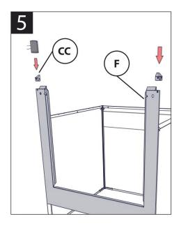
Slide front panel onto corner brackets. Insert the last 2 caps. If you have >1.6m wide models, see step 6 before inserting caps.
