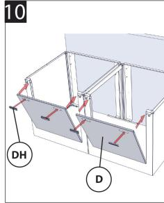
Insert the handles into the door untill a door into the panel by placing the lip of the door over the front panel step. Insert centre hinge pin through both top lids the door by aligning the studs on the side and corner caps. with the slots in the front panel. Push in slightly and then down.
