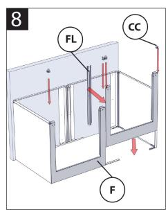
Slide the front panels into position and insert the filler and caps.
