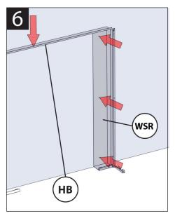
Slide the wall strip onto the corner bracket and attach to wall using appropriate fixings.
