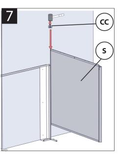
Slide the side panels into position and insert the filler and caps.
