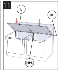
Attach lids to the unit with hinge pins. "click" is heard. Place the removable front Align pins with holes and tap into place with a mallet. For the central join, tap the
