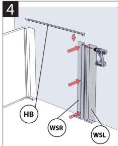
Now insert the other wall fixing strips onto the tabs of the corner and straight brackets.
