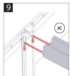
Now it's time to attach the joint channel into the wall strips and front panels. Push tabs into the slots (through fillers and wall strips /front panels) and then push down to lock.
