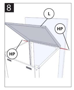
Attach lid to unit with hinge pins. Align pins with holes and tap into place with a mallet. Insert door latches into slots in lid.
