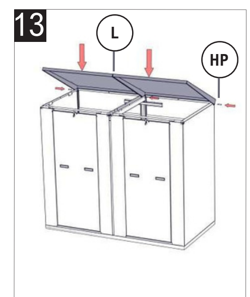
Attach top door to unit with hinge pins. Align pins with holes and tap into place with a mallet.
